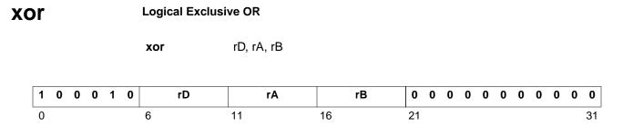
The contents of register rA are XORed with the contents of register rB; the result is placed into register rD.
